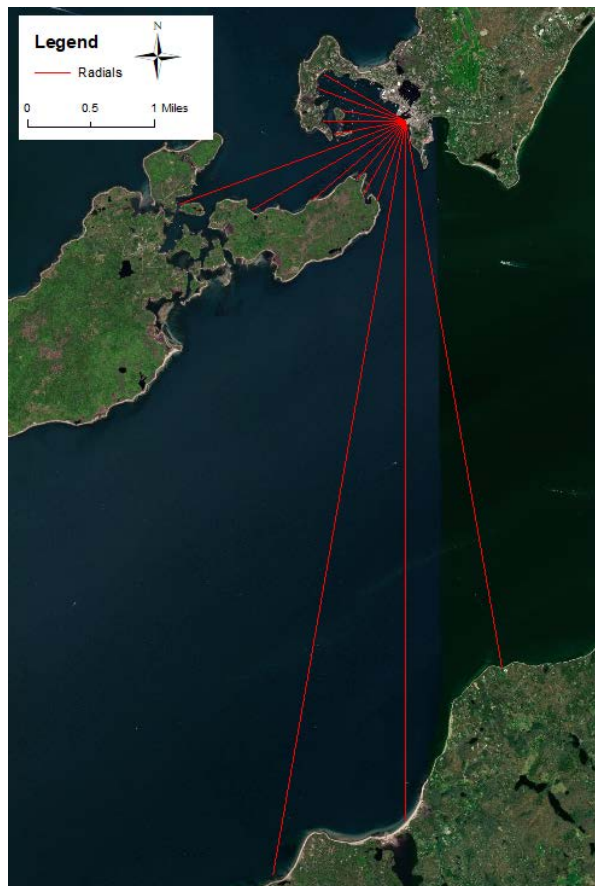
Figure 11: Radials used in ACES to determine the fetch limited wave height at the Woods Hole Ferry Terminal.
